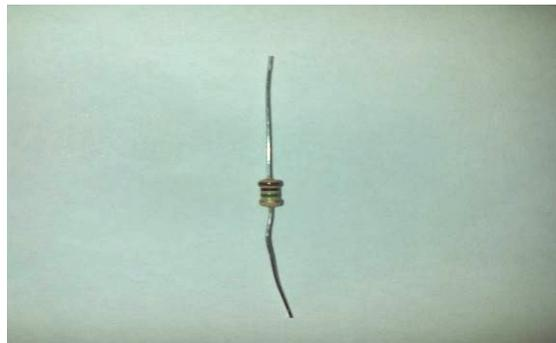
Figura 18: Resistor de  $1M\Omega$ .
